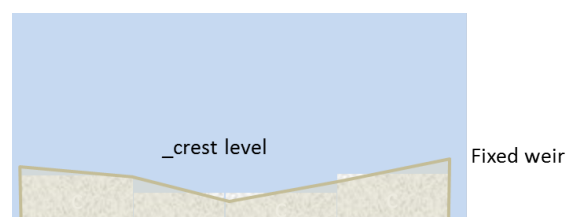
Figure 5.16: Schematic representation of a fixed weir
