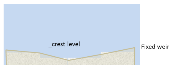
Figure 5.16: Schematic representation of a fixed weir
