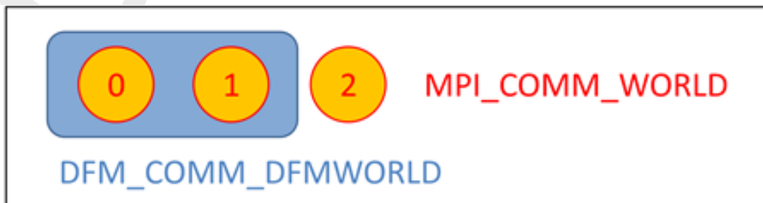
Figure 1.3: In a parallel run using a parallel communicator, DIMR initializes MPI and creates a MPI_COMM_WORLD communicator in DimrExe::initialize_parallel . In Dimr::runParallellnit 2 processes are assigned to “ dflowfm ”, as specified in the configuration file snippet shown above. Note that DFM_COMM_DFMWORLD is part of MPI_COMM_WORLD .
