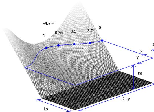
Figure 3.4: Definition sketch of concave beach bathymetry
