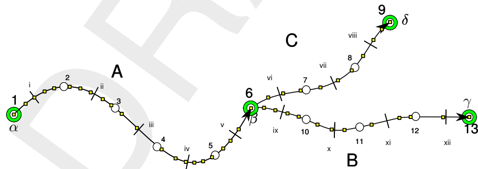
Figure 1: Simple computational 1D network; 3 branches (A, B, C), 4 network nodes (green circles, \alpha , \beta , \gamma , \delta ); 13 nodes (open circles + green circles, \zeta -points, latin numbers), 12 edges ( u -points; roman numbers), 44 network nodes (yellow squares)
